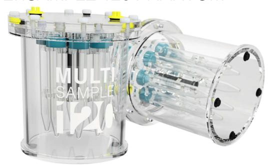
The MultiSample120 phantom is a 120mm diameter cylindrical phantom, capable of holding up to eight industry standard Falcon BD 15ml polypropylene tubes. The phantom can be supplied empty for filling by the user, or can be filled with solutions to the customer's specification. Uses include:
