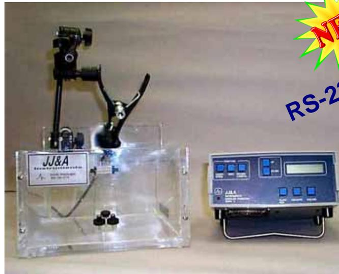
The Mark 4 *Plus* Doppler phantom is a very accurate device for testing Doppler ultrasound scanners. It is especially useful for checking sample volume registration, color registration, directional discrimination, and Doppler velocity accuracy.
